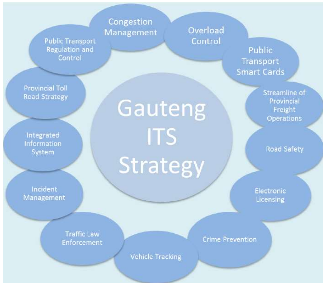
Figure 4-39: The transport subsystems that need to be integrated, as mentioned in the ITS Implementation Framework for Gauteng – 2010
